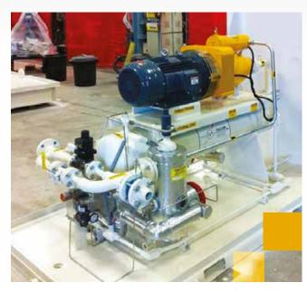
Vapor Recovery Unit (VRU) which uses a Mattei GC 86 gas compressor and a 20HP motor to compresse low pressure Methane Vapor from crude oil tanks and wellheads to higher pressure Methane gas which is then used as a fuel at each site. There are over 100 of these units operating in the Southwest United States.
