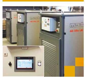
55 kW AG gas compressors used in an installation for an ammonia-based system for removal of CO<sup>2</sup> in Biogas.
