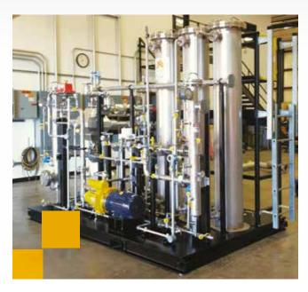
Mattei GC 86 gas end and 15 HP motor installed in a beer brewery to compress brewery waste methane gas to drive a Capstone Micro Turbine to generate electricity used at the site.
